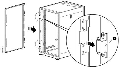
2. Use slight pressure to pull the door away from enclosure; then lower the door
